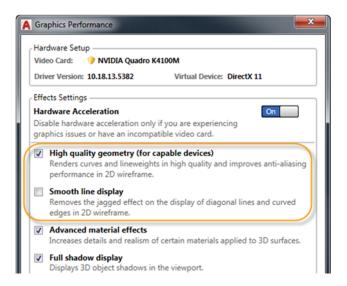
You can access the Graphics Performance dialog box from the Hardware Acceleration tool on the status bar.
