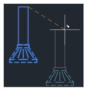
In AutoCAD 2018, the rubber-band line is added to the long list of interface elements for which you can control the color. Access that control from the Colors button on the Display tab of the Options dialog box.
