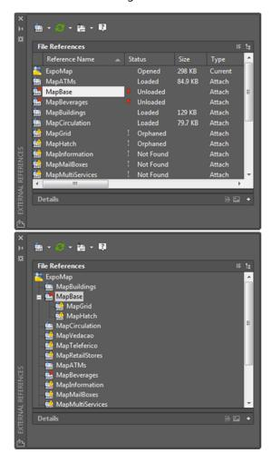
The Open option is no longer disabled when you right-click on an unloaded reference in the External References palette, enabling you to quickly open unloaded reference files.
