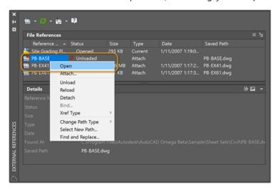
If you rename an unloaded reference in the External References palette, it no longer automatically reloads. It remains unloaded until you intentionally reload it.
