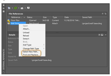
Select New Path allows you to browse to a new location for a missing reference file (fix one), and then provides you with an option to apply the same new location for other missing references (fix all).
