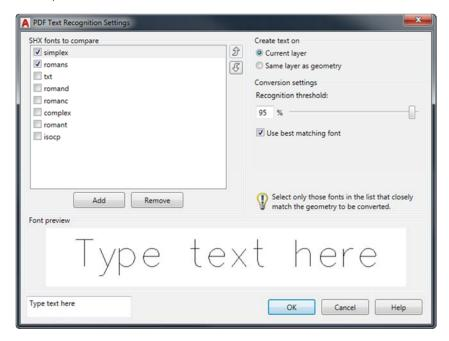
After comparing the geometry to the SHX fonts, the geometry that matches is automatically replaced with one or more Mtext objects. A message box will display the results.
