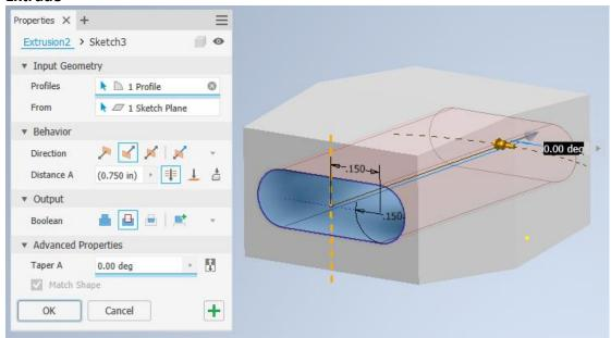
When using the taper option with adjacent regions, the operation merges the faces to create a single, unified result.
