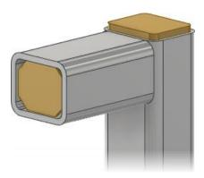
Use the new Insert End Cap command to close structural frame members. You can set the position, thickness, specify the profile shape, other properties.
